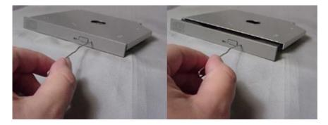
Figure 2.Using Emergency Eject
